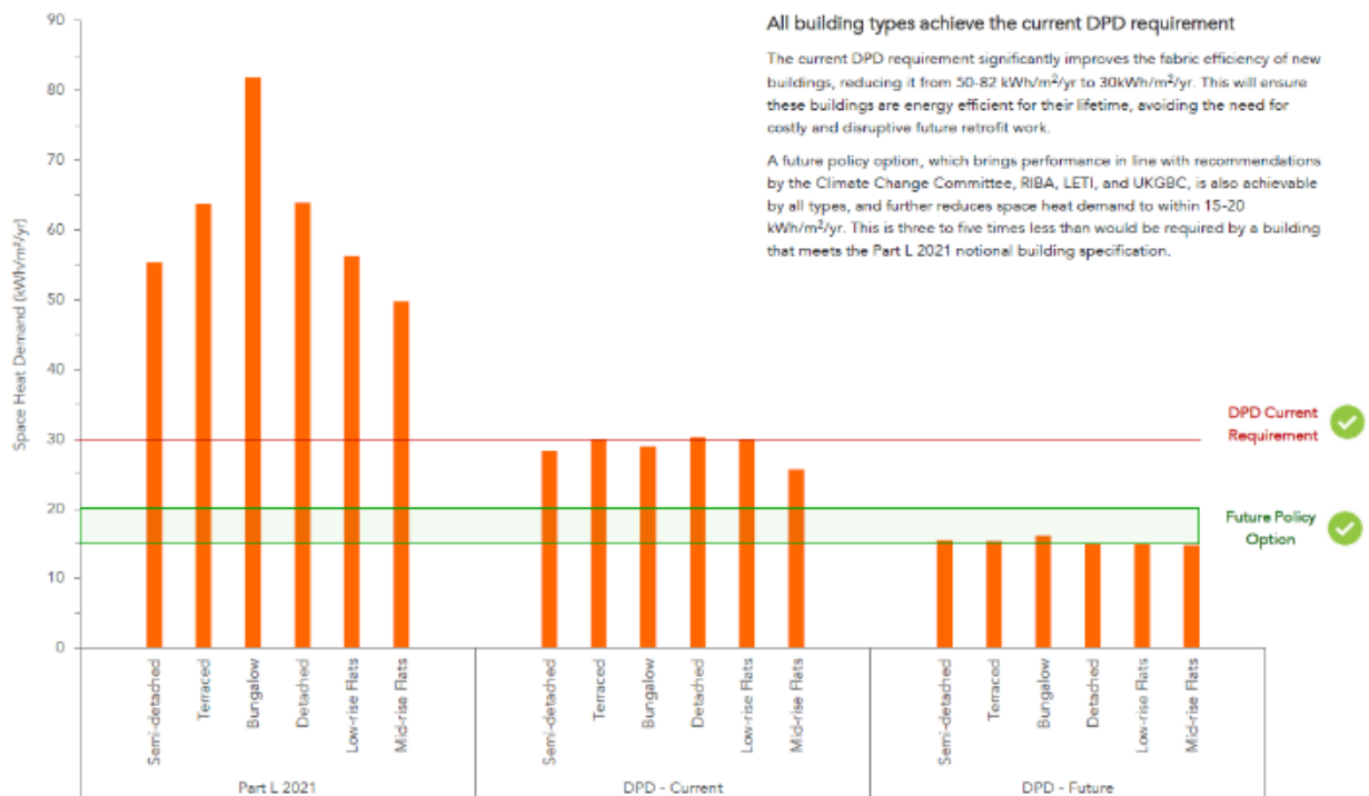
Figure 4: space heating performance of the six residential typologies assessed by Cornwall all able to meet stretching targets of 15-20 kWh/m 2 /yr
