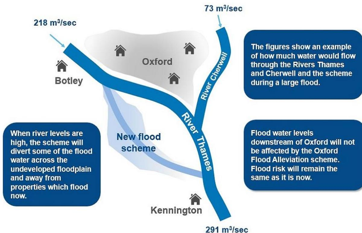
Figure 12- Schematic of Oxford Flood Alleviation Scheme<sup>28</sup>
