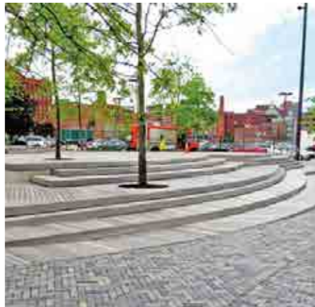
Varied use of permeable paving surfaces with flow control creates visual interest
