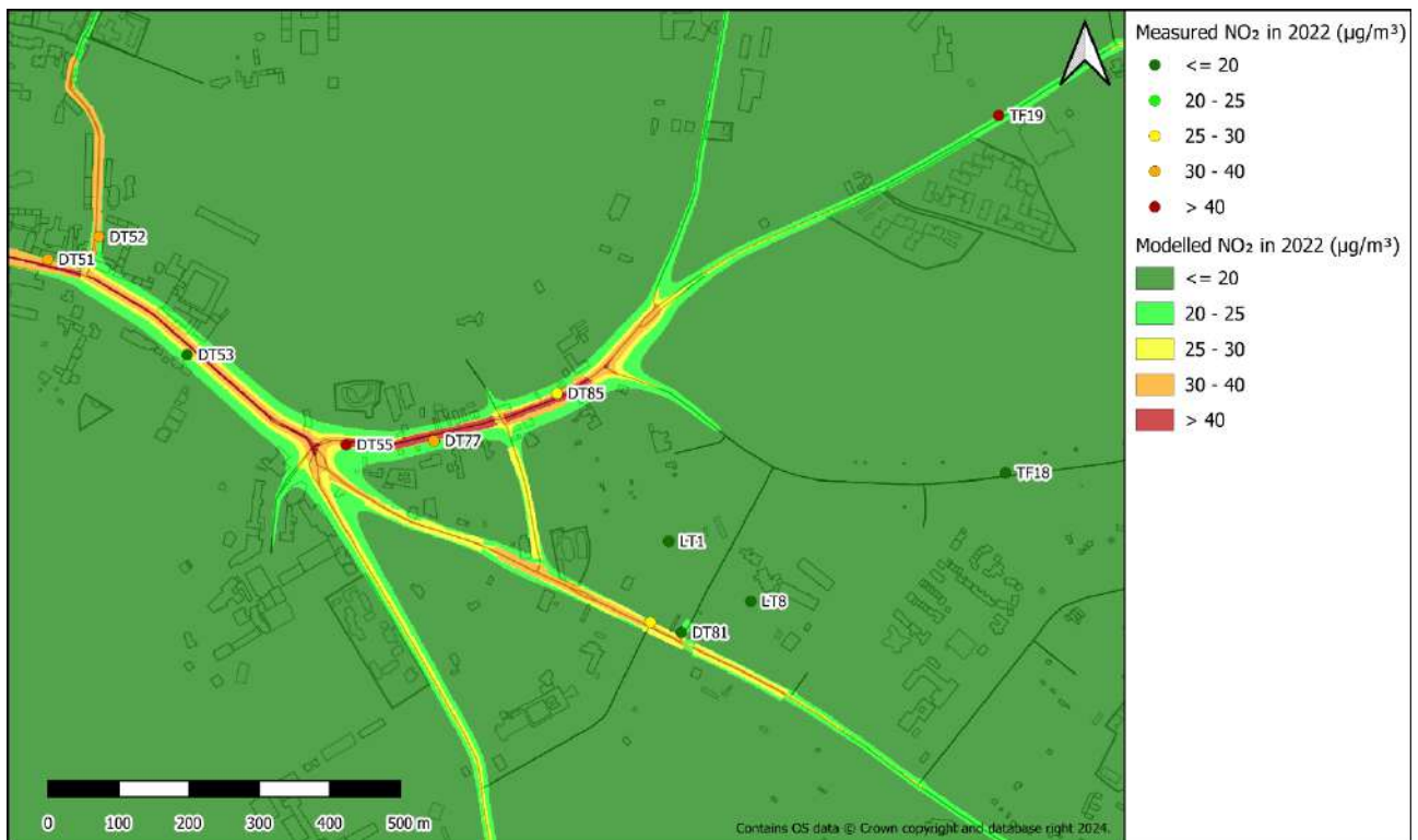
Figure 3-2 Baseline model results and measured NO 2 in 2022 at St Clements/ The Plain.
