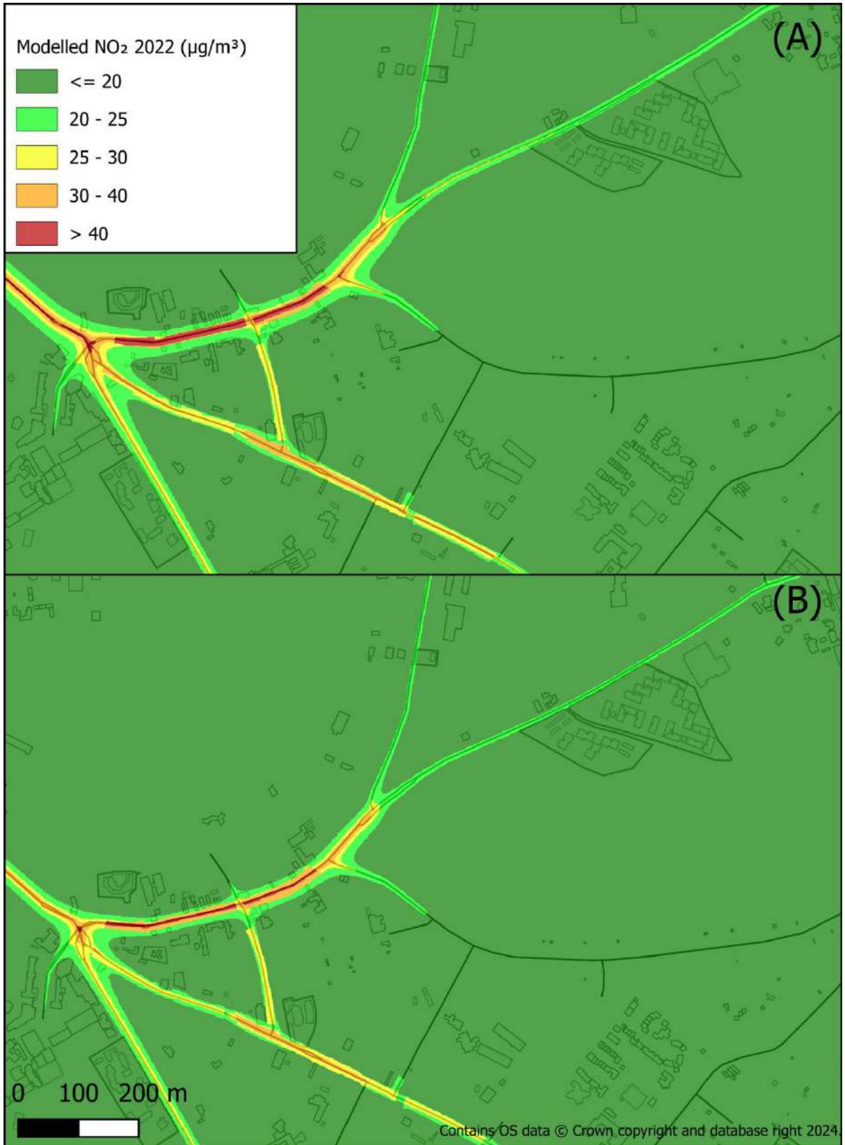
Figure 4-3 Modelled total NO 2 concentrations (2022) at St Clement's / The Plain using (A) a baseline fleet and (B) the ZEBRA fleet in which 69% of buses are zero emission.
